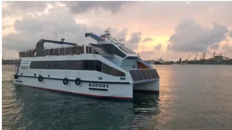
The catamaran is primarily powered by a 40 kW IVECO Marine Diesel generator, which provides propulsion and backup energy. To reduce emissions, a 4.4 kWp photovoltaic system was installed in 2021, consisting of 10 Longi 370 Wp modules and 4 Victron Energy 175 Wp modules. This system powers essential onboard loads, including navigation equipment, lighting, and communication systems. Over three years, it produced 9 MWh of
