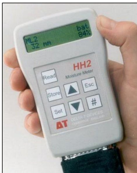
Figure 2. HH2 moisture meter
